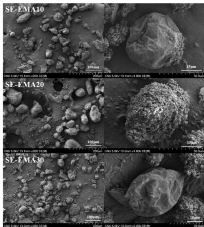
**Figure 6.** SEM images of the microcapsules prepared with the input of different weight portion of comonomer EMA through suspension polymerization.
