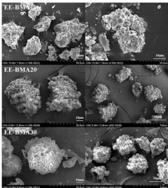
**Figure 11.** SEM images of the microcapsules prepared with various weight portions of comonomer BMA through emulsion polymerization.
