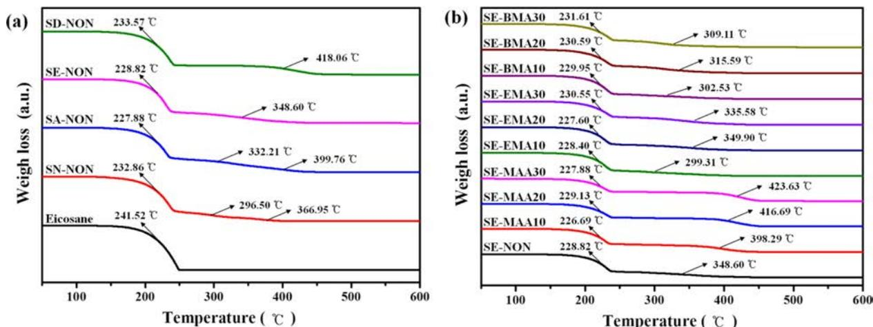
**Figure 16.** TGA thermograms of the microcapsules prepared by suspension polymerization with various crosslinking agents (a) and comonomers (b) differing in their weight portions.
