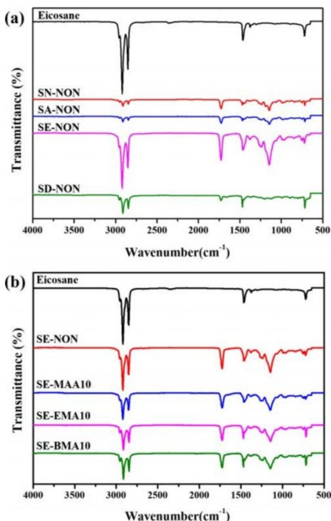
**Figure 2.** FTIR spectra of the microcapsules prepared by suspension polymerization with different crosslinking agents (a); different acrylic comonomers (b).
