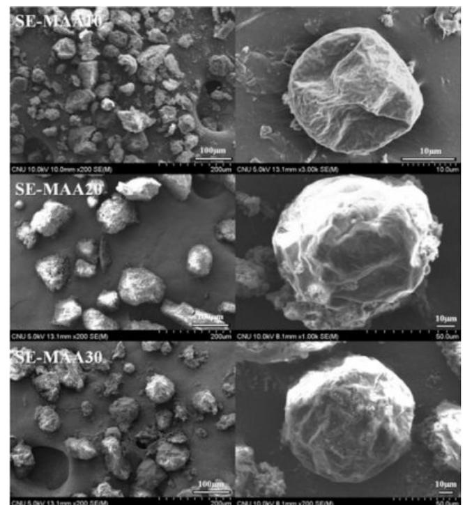
**Figure 5.** SEM images of the microcapsules prepared with the input of different weight portion of comonomer MAA through suspension polymerization.
