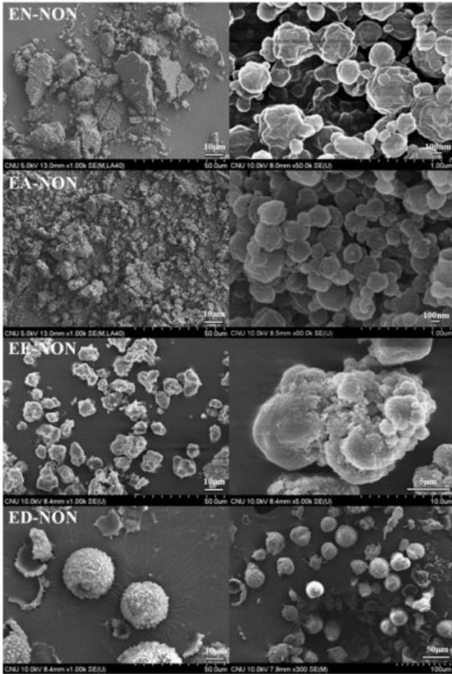
**Figure 8.** SEM images of the microcapsules prepared by emulsion polymerization with various crosslinkers.
