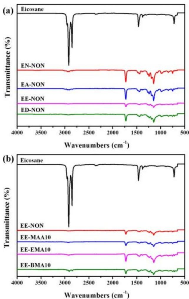
**Figure 3.** FTIR spectra of the microcapsules prepared by emulsion polymerization with different crosslinking agents (a); different acrylic comonomers (b).
