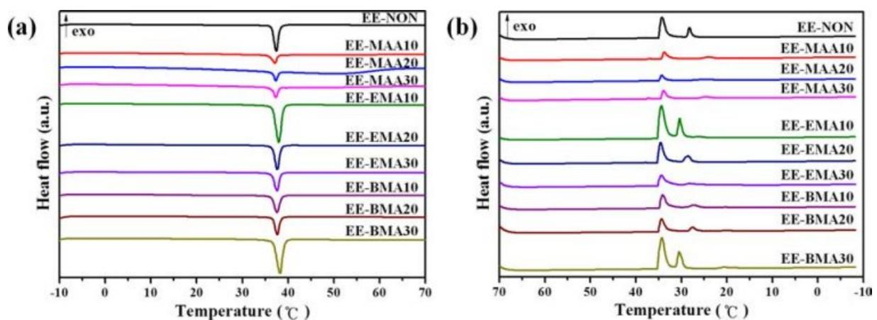
**Figure 15.** DSC heating (a); cooling (b) thermograms of microcapsules prepared by emulsion polymerization using various comonomers with various compositions.
