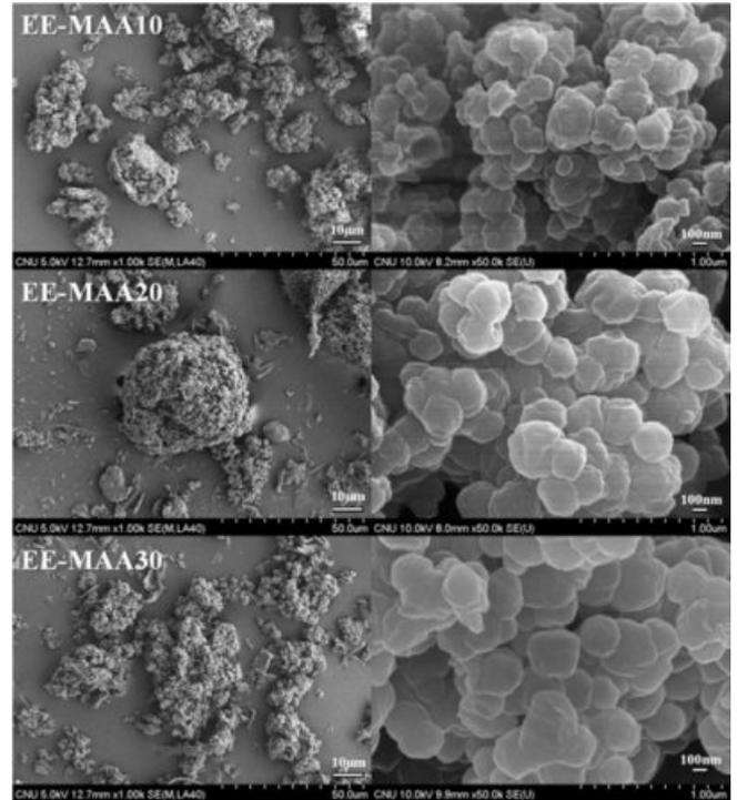
**Figure 9.** SEM images of the microcapsules prepared with various weight portions of comonomer MAA through emulsion polymerization.
