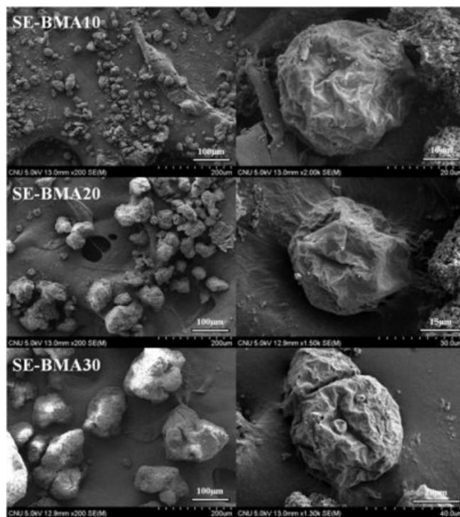
**Figure 7.** SEM images of the microcapsules prepared with the input of different weight portion of comonomer BMA through suspension polymerization.
