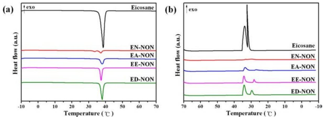
**Figure 14.** DSC heating (a); cooling (b) thermograms of microcapsules prepared by emulsion polymerization using various crosslinking agents.
