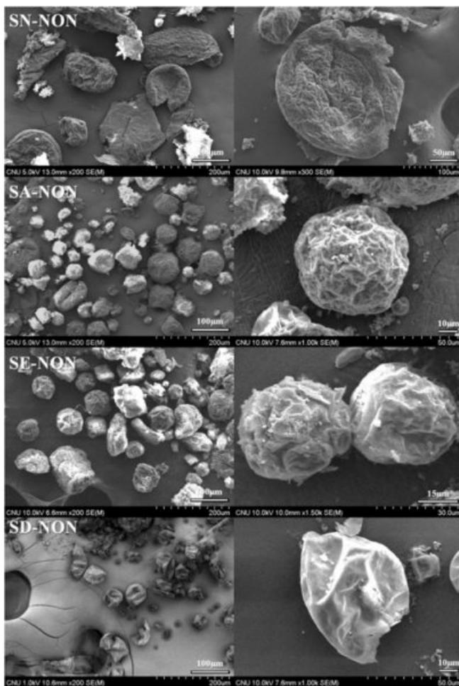
**Figure 4.** SEM images of the microcapsules prepared by suspension polymerization with various crosslinkers.
