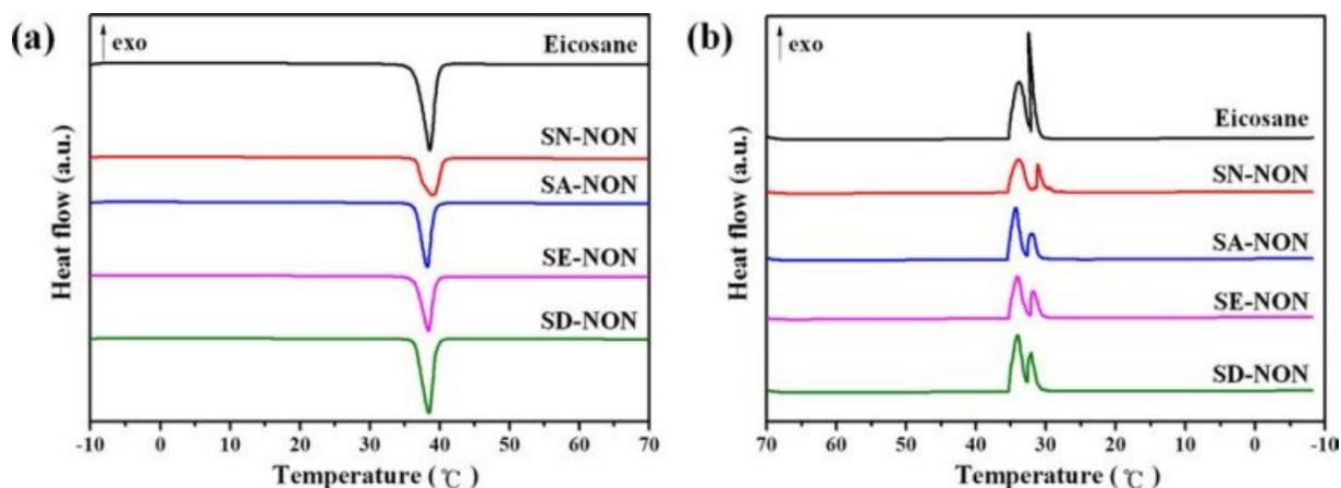
**Figure 12.** DSC heating (a); cooling (b) thermograms of microcapsules prepared by suspension polymerization using various crosslinking agents.
