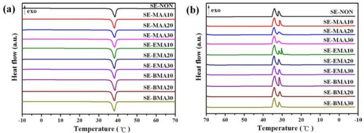
**Figure 13.** DSC heating (a); cooling (b) thermograms of microcapsules prepared by suspension polymerization using various comonomers different in their weight portions.
