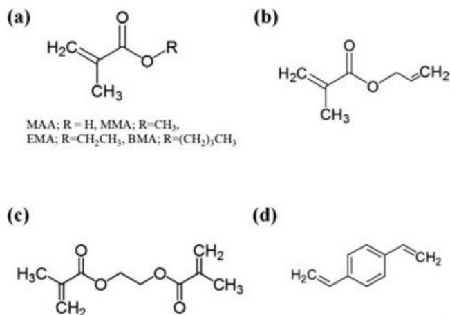
**Figure 1.** Chemical structures of acrylic monomers and crosslinking agents used in this study: (a) MAA; MMA; EMA; BMA; (b) AMA; (c) EGDMA; (d) DVB.
