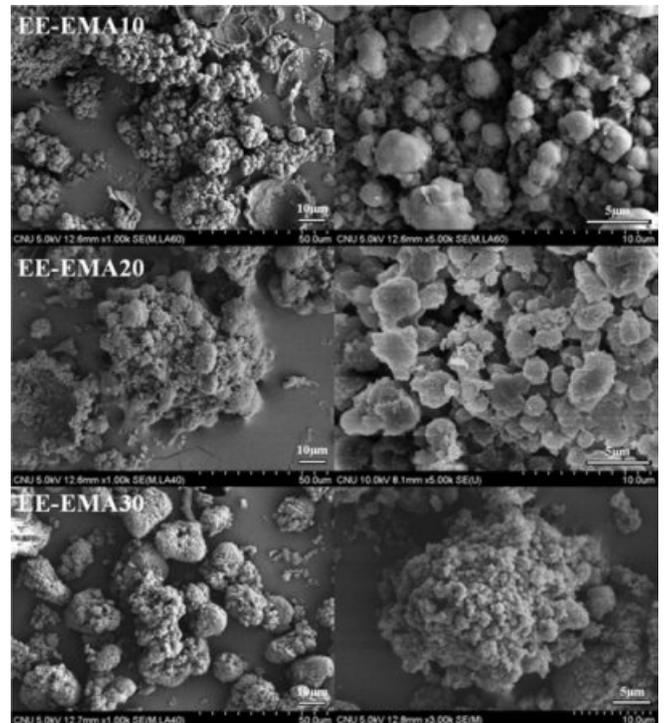
**Figure 10.** SEM images of the microcapsules prepared with various weight portions of comonomer EMA through emulsion polymerization.
