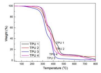
Figure 1. TGA results of TPU samples.
