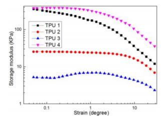
Figure 5. Storage modulus of TPU samples.
