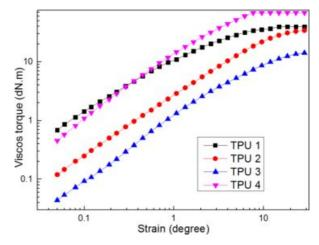
Figure 9. Viscous torque of TPU samples.
