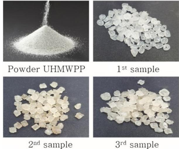
**Figure 8.** Pellet shape according to number of extrusions.
