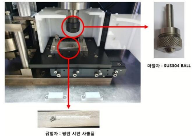
**Figure 2. Dynamic friction coefficient measurement equipment.**
