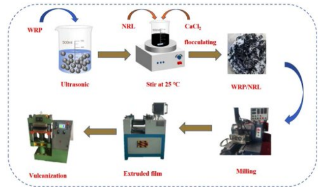
Figure 2. Preparation process of vulcanized rubber.
