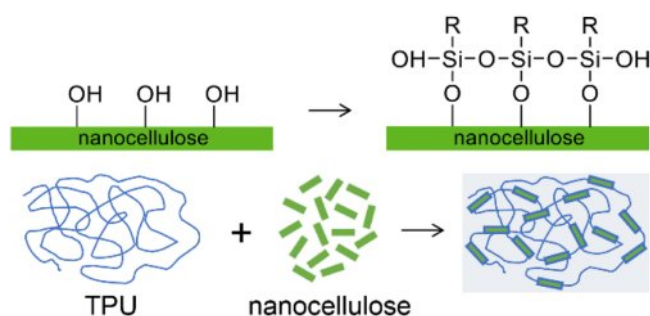
Scheme 1. Scheme of surface modification of CNC by silane coupling agents and fabrication of TPU composite. R represents -(\text{CH}_2)_3\text{NH}_2 for APTES and -(\text{CH}_2)_7\text{CH}_3 for OTES.
