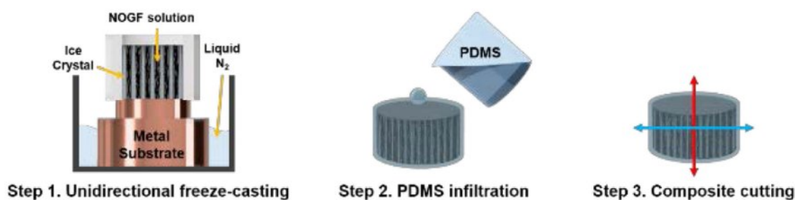
Figure 2. Schematic illustration of fabrication process for the composites prepared in this study.
