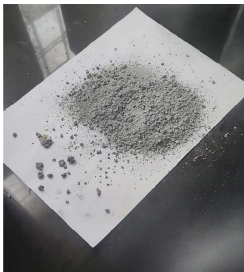
Figure 7. The shape of the 20 phr CaO MPU composite after sieving.
