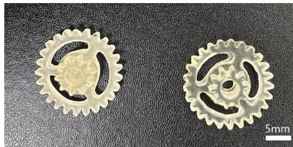
Figure S3. Image of gears that were printed using UTIS1 (left) and UTIS2 (right).
