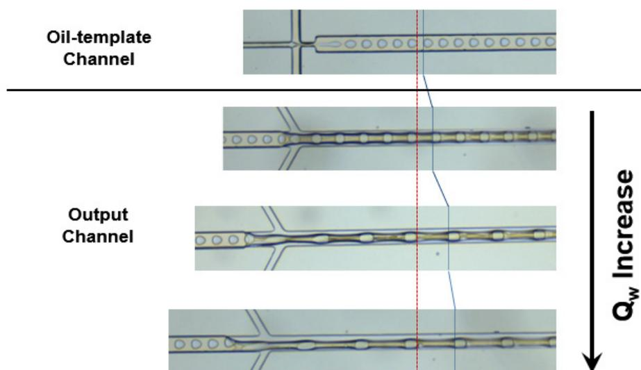
**Figure. S1.** Optical microscope images of the generation of oil droplets in the oil-template channel and cellulose fibers in the output channel. From the top to the bottom images, the flowrate of the aqueous phase ( $Q_w$ ) in the output channel was 1.7, 3.3, and 5.0  $\mu\text{L min}^{-1}$ , respectively; the ratio of the flowrates of the oil and cellulose-containing EMIM-Ac ( $Q_{\text{oil}}/Q_{\text{c-IL}}$ ) was fixed at 0.3.
